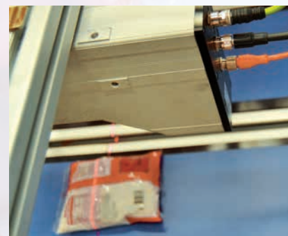
IVC-3D provides three-dimensional position data and timing information.
