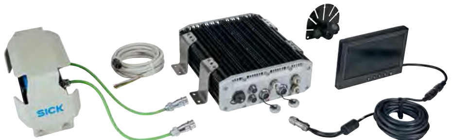
The Visionary-B CV is based on the stereoscopic principle, which is similar to the way that humans perceive space.
