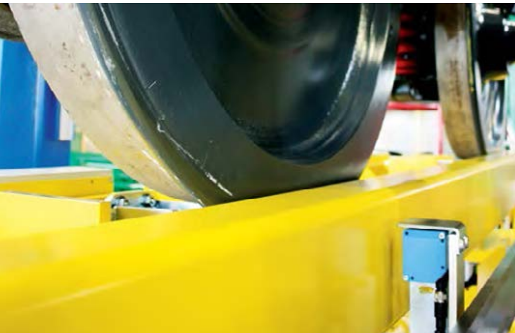
Displacement measurement sensors in action.
