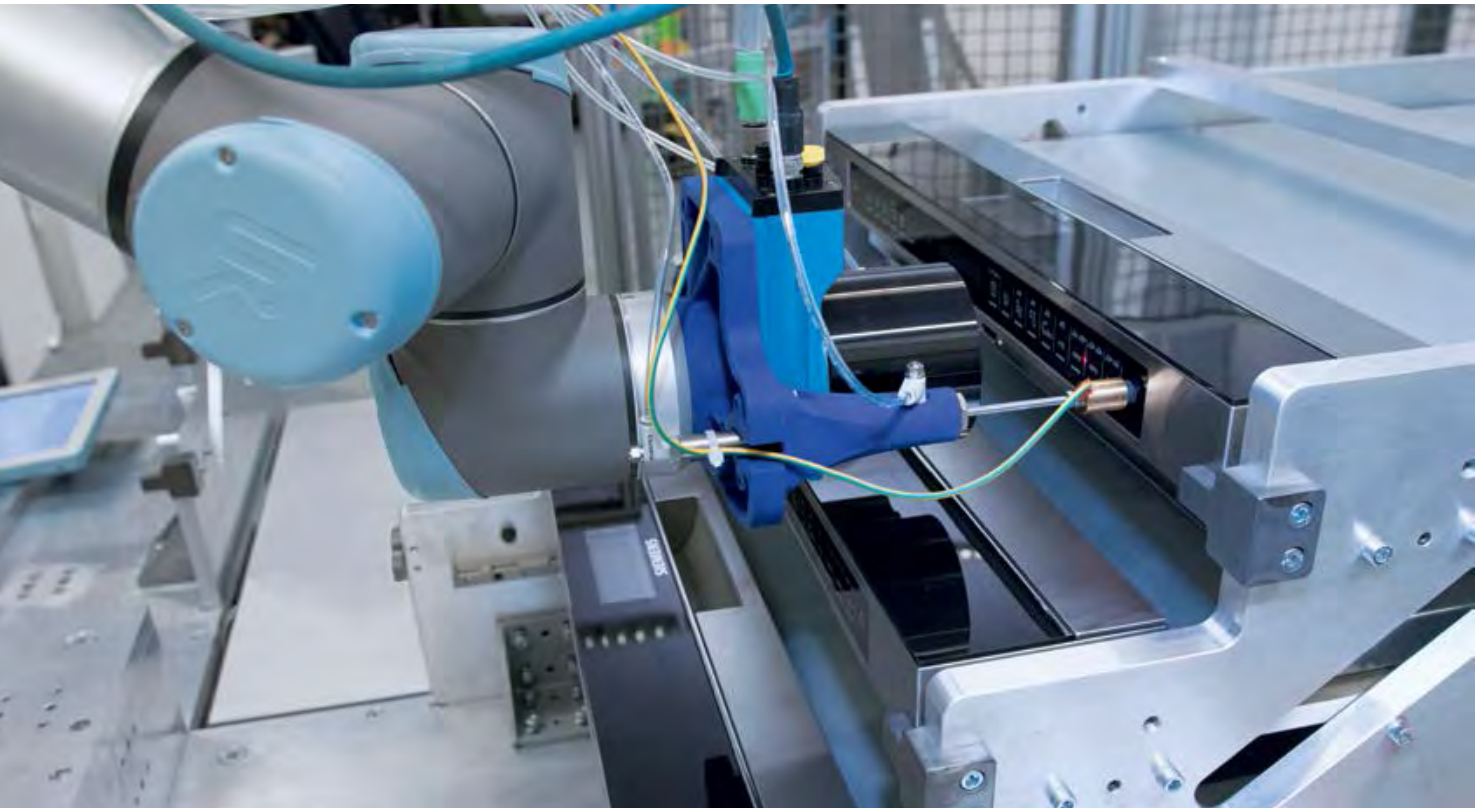
The robot uses the testing fingers on its arm to check each individual key on the dishwasher control panel.
