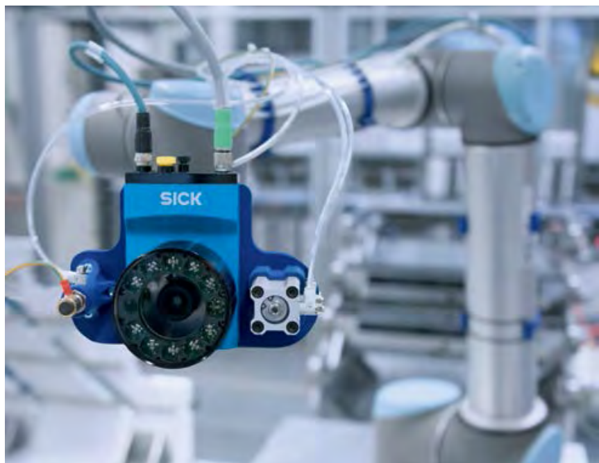
The programmable 2D InspectorP65x camera actively controls the robot arm.
