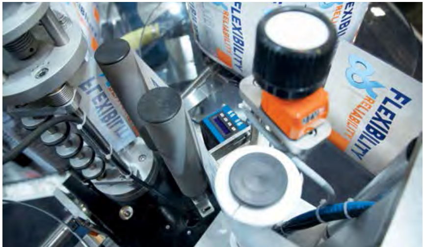
The PS30 really plays to its strengths in presence monitoring applications and when identifying the position of labels, packaging material, or tubes.
