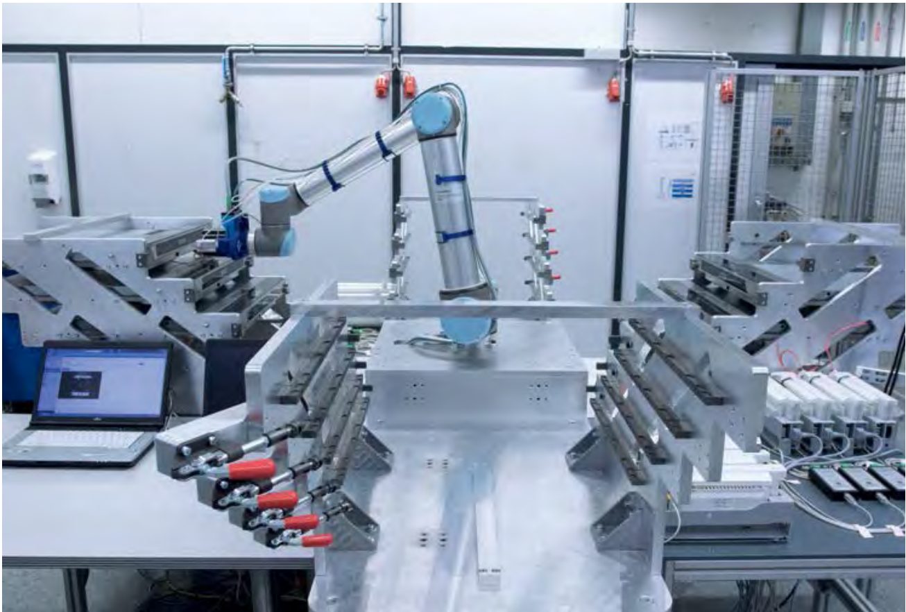
Test lab for conducting lifecycle tests on dishwasher control panels: Mobile robot system conducts entire test cycles.
