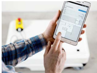
The MiR100 can be controlled using a tablet, cell phone, or PC.
