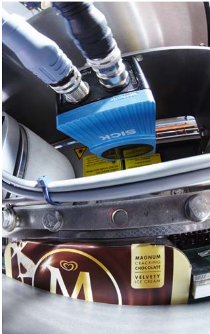
The vision sensor verifies that the use-by date is there.
