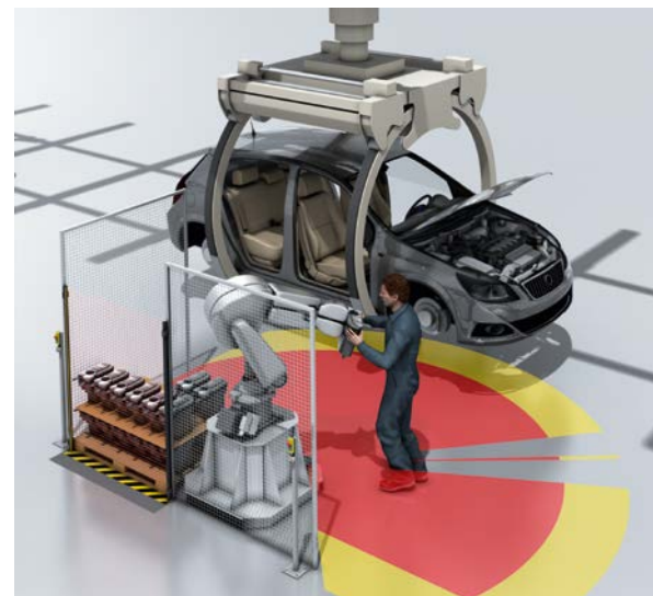
Robots are already able to operate without being surrounded by a safety fence.
